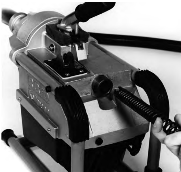
Figure 5 – Inserting Cable Into Front Of Machine
