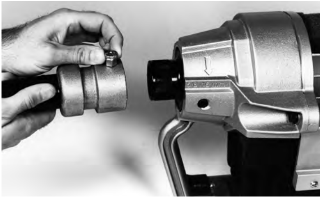
Figure 4 – Rear Guide Hose Attachment
