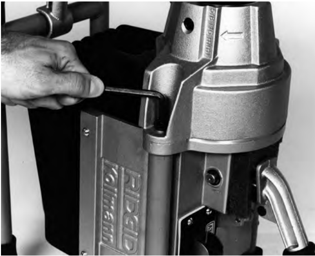
Figure 11 – Remove Socket Head Cap Screws
